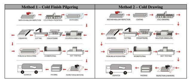
The manufacturing process for seamless tubes and pipes is a well calibrated process in line with applicable industry standards in India. A brief description of the step-by-step manufacturing process (for both the methods as indicated above) is provided below:
