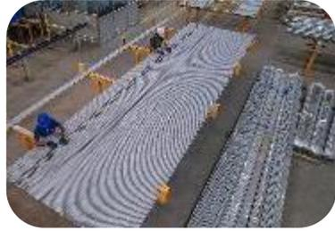
Stainless Steel Hydraulic and Instrumentation Tubes
