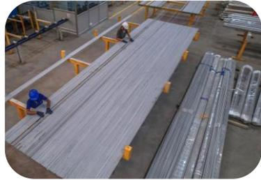
Stainless Steel Hydraulic and Instrumentation Tubes
